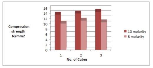
Figure 3. Chart of Compressive Strength for Curing of Geopolymer Concrete Cubes for 28 Days
