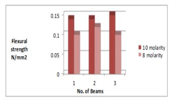
Figure 1. Chart of Flexural Strength of Geo polymer Concrete Beam for 28 Days
